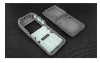
Printing the whole set of radiotelephone parts with PA12 and Flexa Grey costs less than 600 USD and takes about four days. Comparing it to 40 000 USD for the molds used for prototyping purposes the ROI is achieved during the first project. In the end it is the fastest and the most cost-effective solution when precision, detail and surface quality matter.
